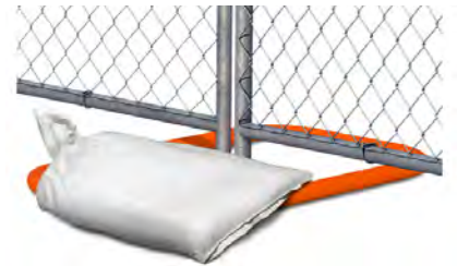
TEMPORARY CHAIN LINK FENCE WITH SAND BAGS
