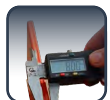
FEET THICKNESS TEST
